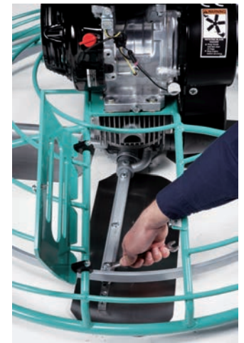
Access panel for quick and easy servicing of trowel arms and blades.
