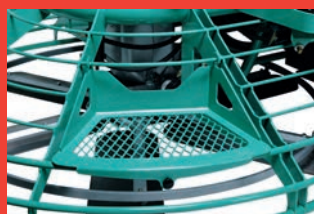
Removable steps provide quick access to trowel blades
