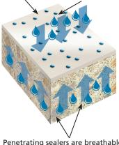
Penetrating sealers are breathable and allow moisture in cured concrete to escape. This reduces the risk of rebar corrosion
